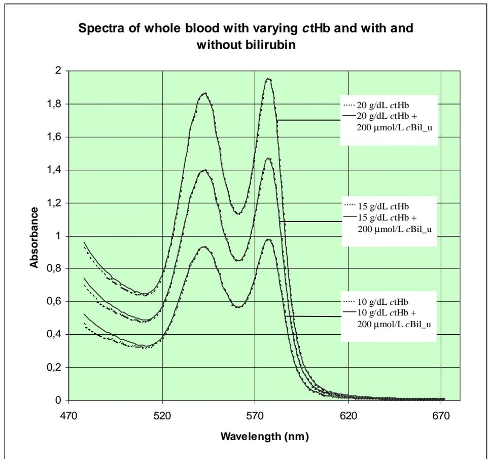
It can be seen in the above diagram that the higher the tHb level is, the less the difference in the spectra when bilirubin is added, and thereby the greater the measurement uncertainty. This illustrates the constraints described above.
