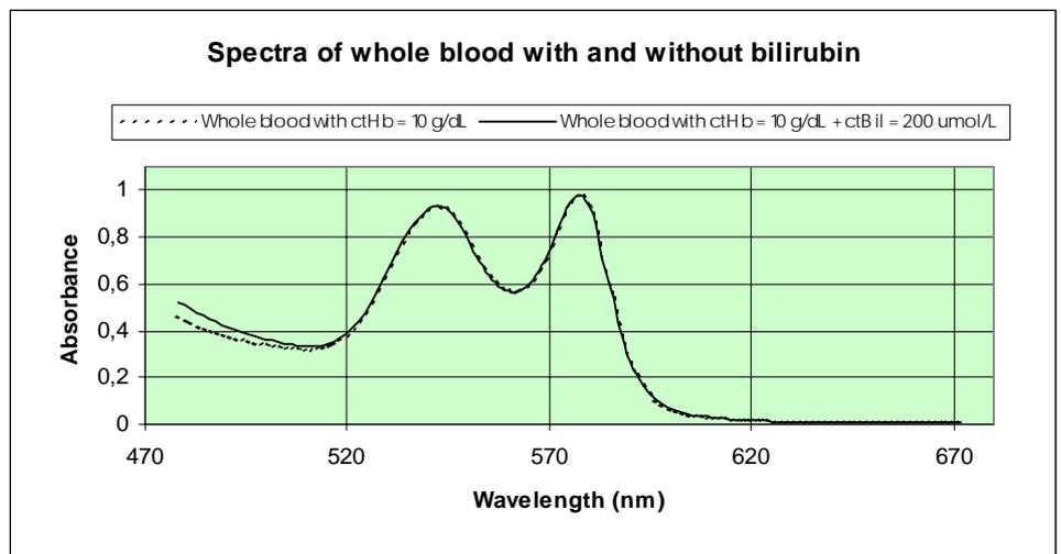
It is the difference in the two spectra, seen between about 478 and 500 nm, which enables us to measure the bilirubin content in whole blood samples.
